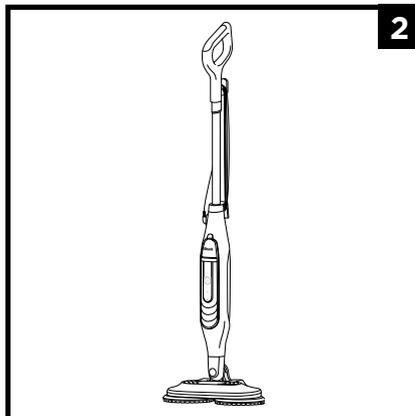
**2** After the unit has cooled and the steam has been released, empty the water tank before storing. Open the tank lid and pour the water out into a sink or bath. After all the water has drained out, close the lid.
