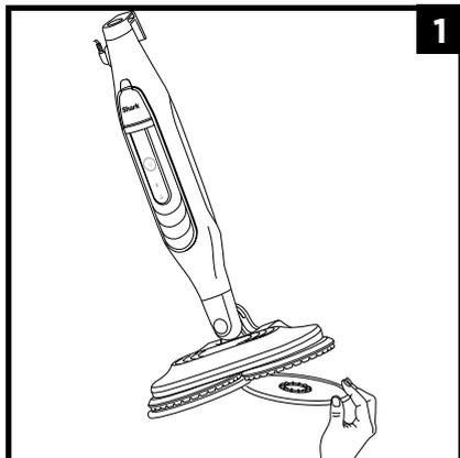
**1** When the pads have cooled completely, remove them by pulling them off the discs.
