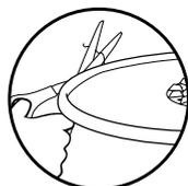
Loose fibres can indicate wearing of the microfibre fabric. **DO NOT** pull the loose fibres as this can cause the weave to come undone. Simply trim the loose fibres with scissors.
